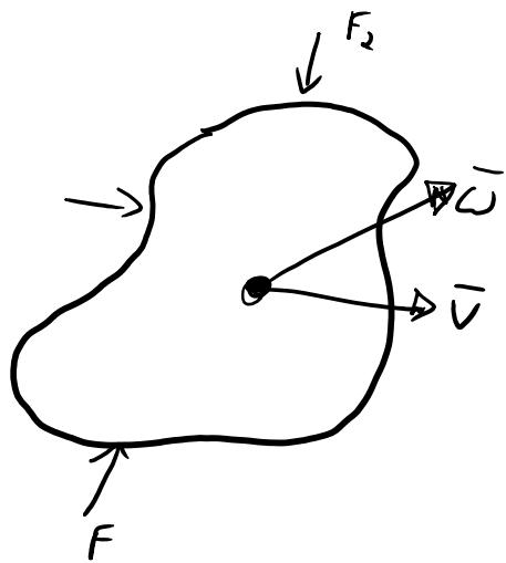
$$\bar{V}_Q = \bar{V}_0 + \bar{\omega} \times \bar{r}^{O \rightarrow Q} = \bar{V}_0 + \bar{\omega} \times (\bar{r}^{O \rightarrow P} + \bar{r}^{P \rightarrow Q})$$
