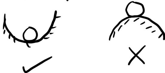
For the aircraft the horizontal tail is the key piece to provide static stability, (why it is also called the "stabilizer".)
