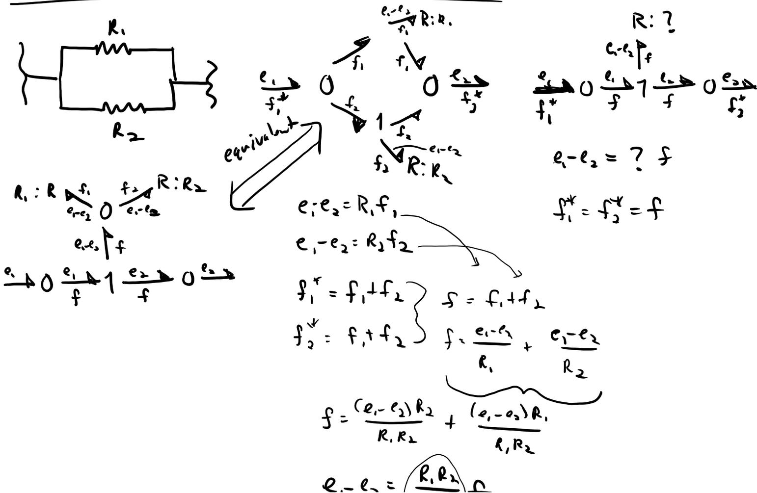
$$e_1 - e_2 = \frac{R_1 R_2}{R_1 + R_2} f$$
