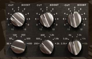
**EQ** Each Channel has its own set of three bell-type filters. The knob on the bottom selects the frequency, the knob above boosts or cuts as desired with a range of +/- 12dB. By default, the plugin operates in Stereo mode, so a change on one channel will be mirrored on the other.
