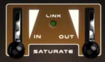
**DUAL TRANSFORMERS** Novatron is the first compressor we know of — analog or plugin — to offer fully controllable Transformer Saturation on both the Inputs and the Outputs. This allows the operator to shape the tone and transients before compression, making them rounder and easier to control, as well as after compression, where they can be further softened and thickened. Either or both Saturation stage can be driven into
