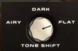
**TONE SHIFT** Use this rotary switch to choose between 2 switchable pre- and post-compression emphasis circuits — Dark, with a gently rolled-off 525-ish vibe, and Airy, with a softly present La2a sparkle — along with 'Flat', which defeats the tone circuit entirely and allows for more neutral processing when desired.
