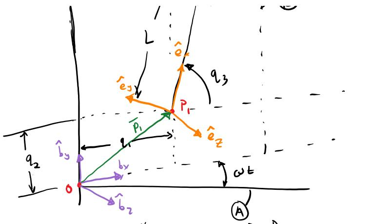
$$\begin{aligned} {}^A \bar{\alpha}_{P_i} &= {}^B \bar{\alpha}_{P_i} + {}^A \bar{\alpha}^{B/A} + 2 \omega {}^B \bar{v} \times {}^B \bar{v}_{P_i} \\ {}^A \bar{\alpha}_{P_i} &= \underbrace{{}^A \dot{q}_1 b_x + {}^A \dot{q}_2 b_y}_{\ddot{q}_1 b_x + \ddot{q}_2 b_y} - \omega^2 q_1 b_x - 2 \omega \dot{q}_1 \hat{b}_z \end{aligned}$$
